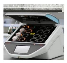
While EPA approval for the TECTA technology currently covers presence/absence of total coliform and E. coli in drinking water, this tool can be utilized in fecal bacteria investigations to determine sources of fecal bacteria contamination as well as disinfection effectiveness. The unit is also mobile and can be easily transported to a facility's on-site laboratory for real-time results
