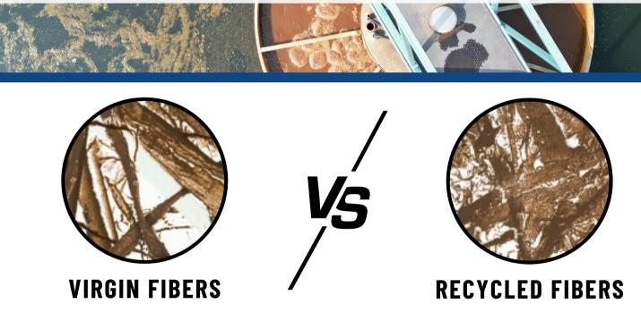
Virgin fibers are longer, stronger, and more easily degraded, making them more efficient for manufacturing. Recycled fibers, on the other hand, are shorter and more contaminated due to previous usage, which makes them harder to degrade in wastewater treatment.
