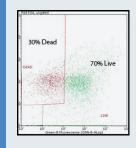
EBS quantifies the total and live bacteria within your system using flow cytometry. This technique is used to better understand how growth pressure stressors impact bacterial activity within a wastewater treatment system.
