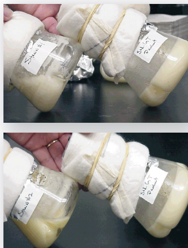
Figures 2 and 3 - Fat degradation capabilities of two LiquiStar GT isolates (left) compared to a commercially available grease trap product.
